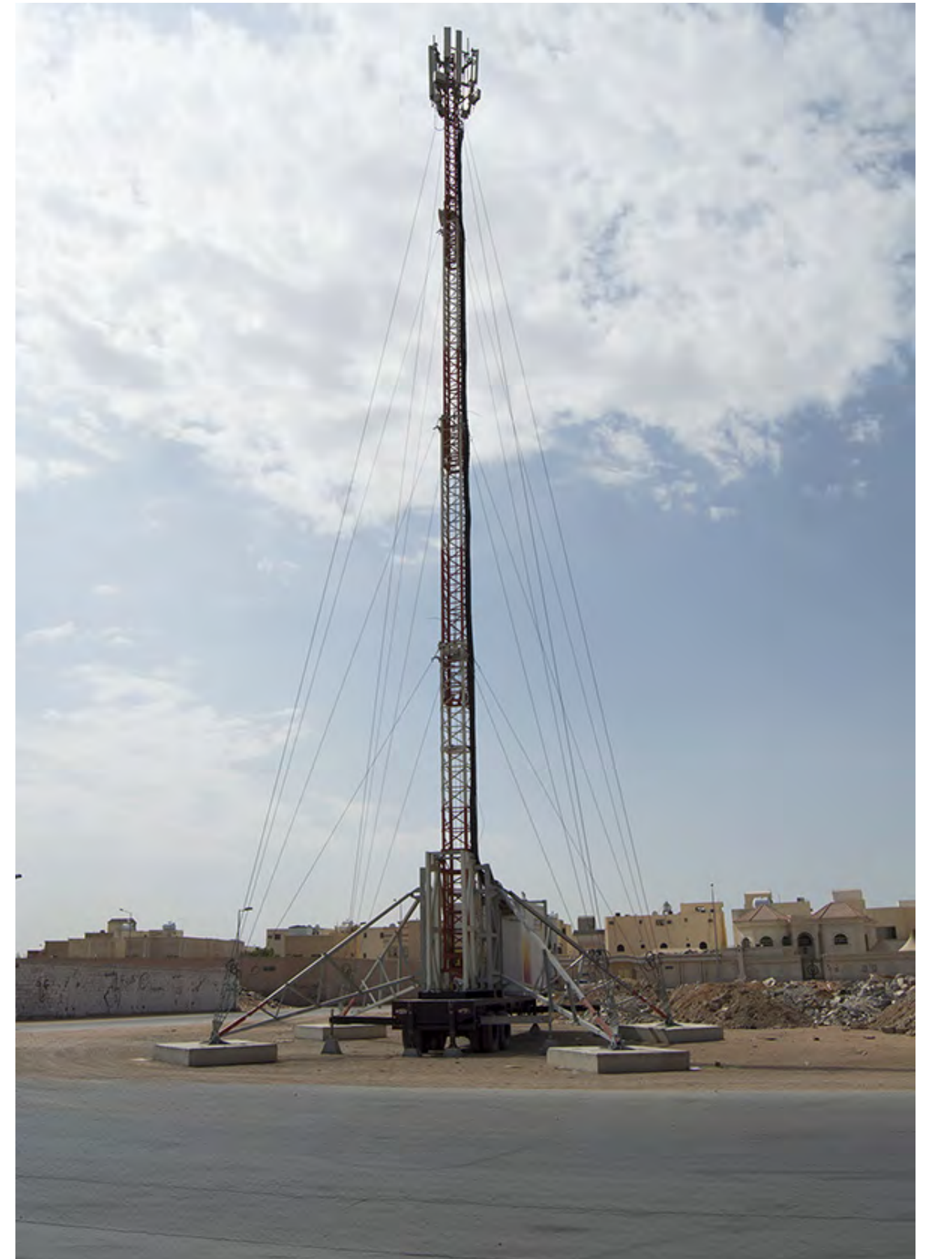
Client: G- Enviro Project: Heavy duty cow GSF Scope: Supply heavy duty cow (trailer with telescopic tower)
