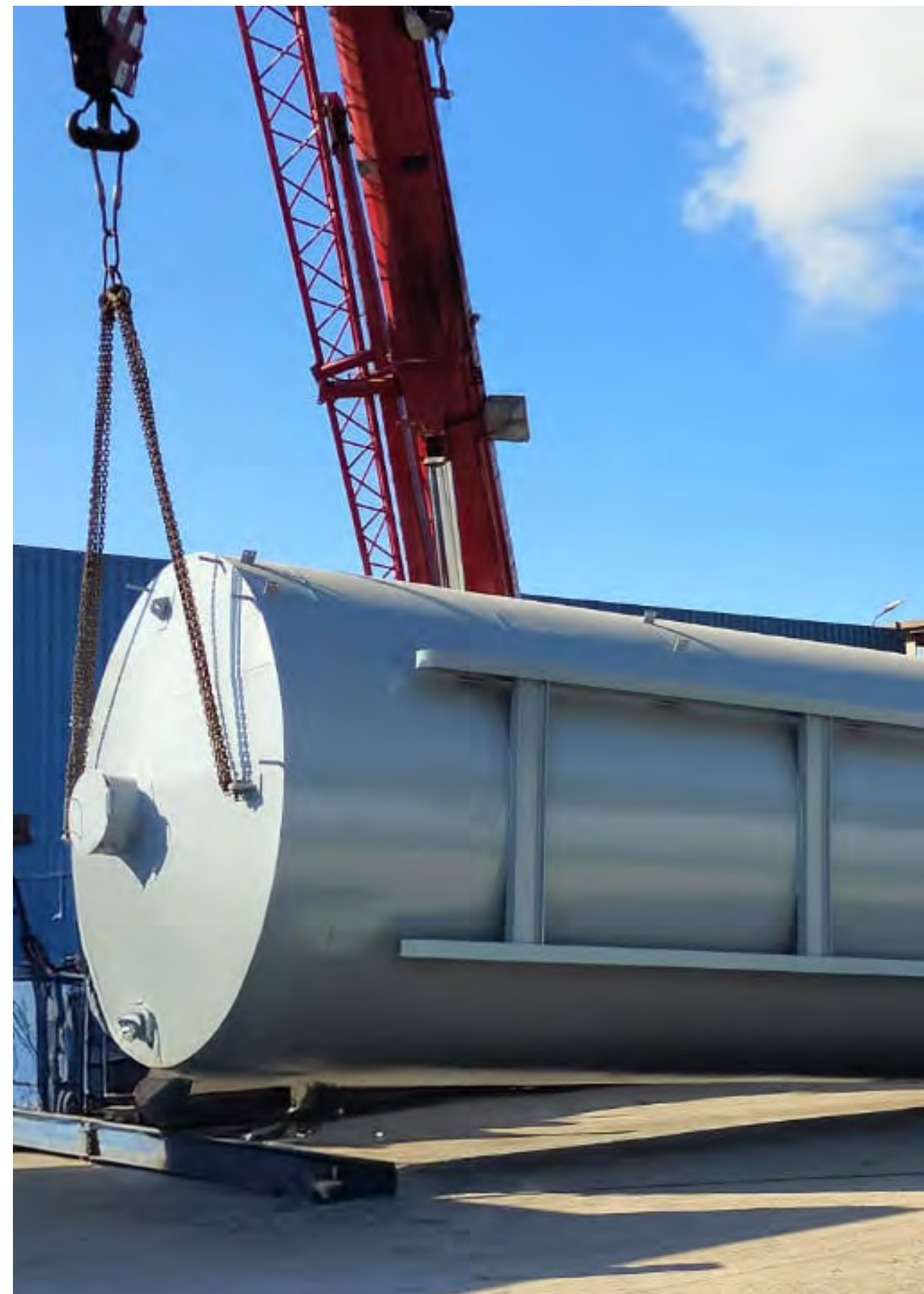
Client: Supplied to Halliburton GSF Scope: Supply, fabrication & epoxy painting of 750 BBL Storage Tanks with handrail and ladder Total Quantity: 110 Tonnes
