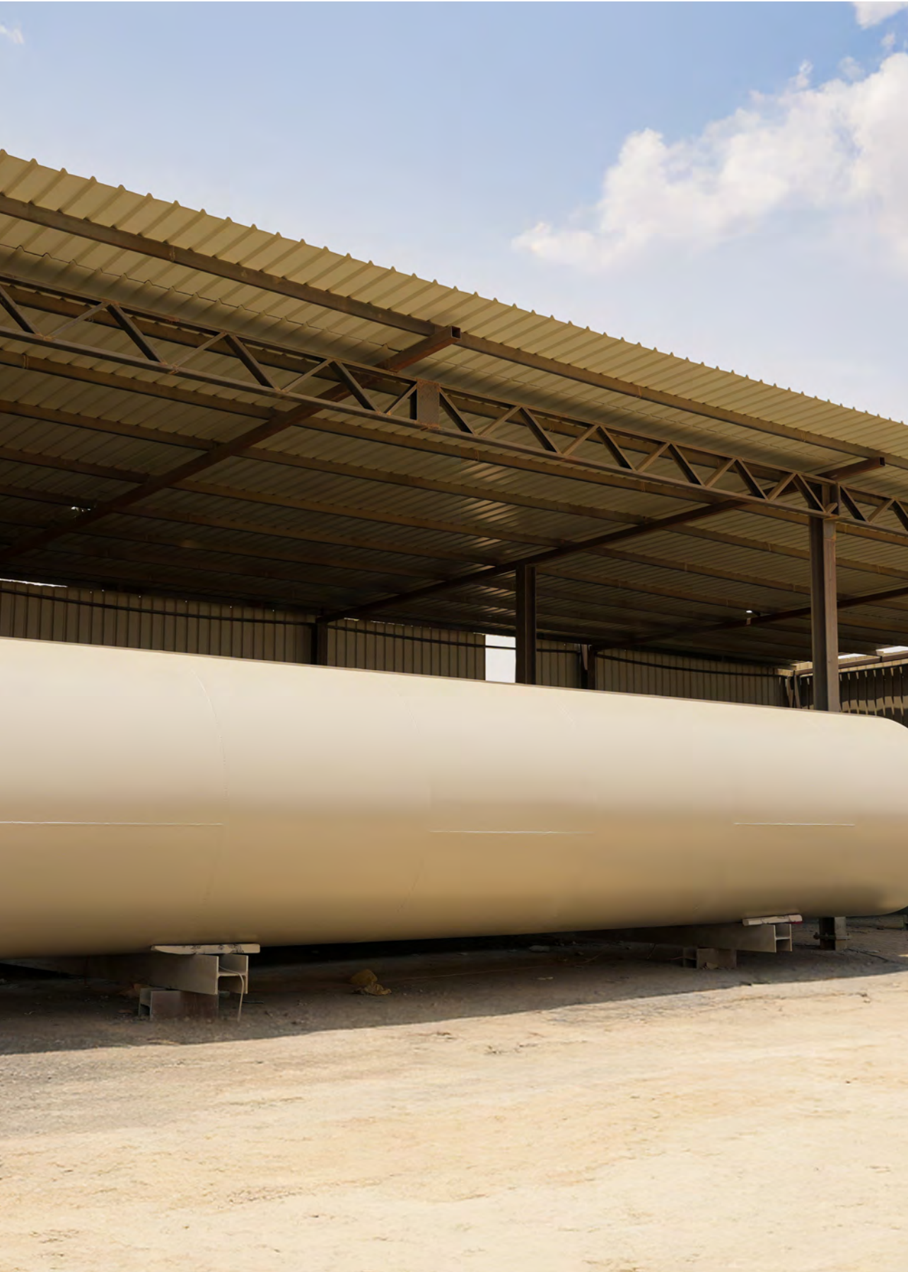
Client: Madkour | Zone: S - TOSKA Booster Pump Stations: DN400 - DN1400 Total Length: 4,224 m | Thickness: 10 mm - 14 mm
