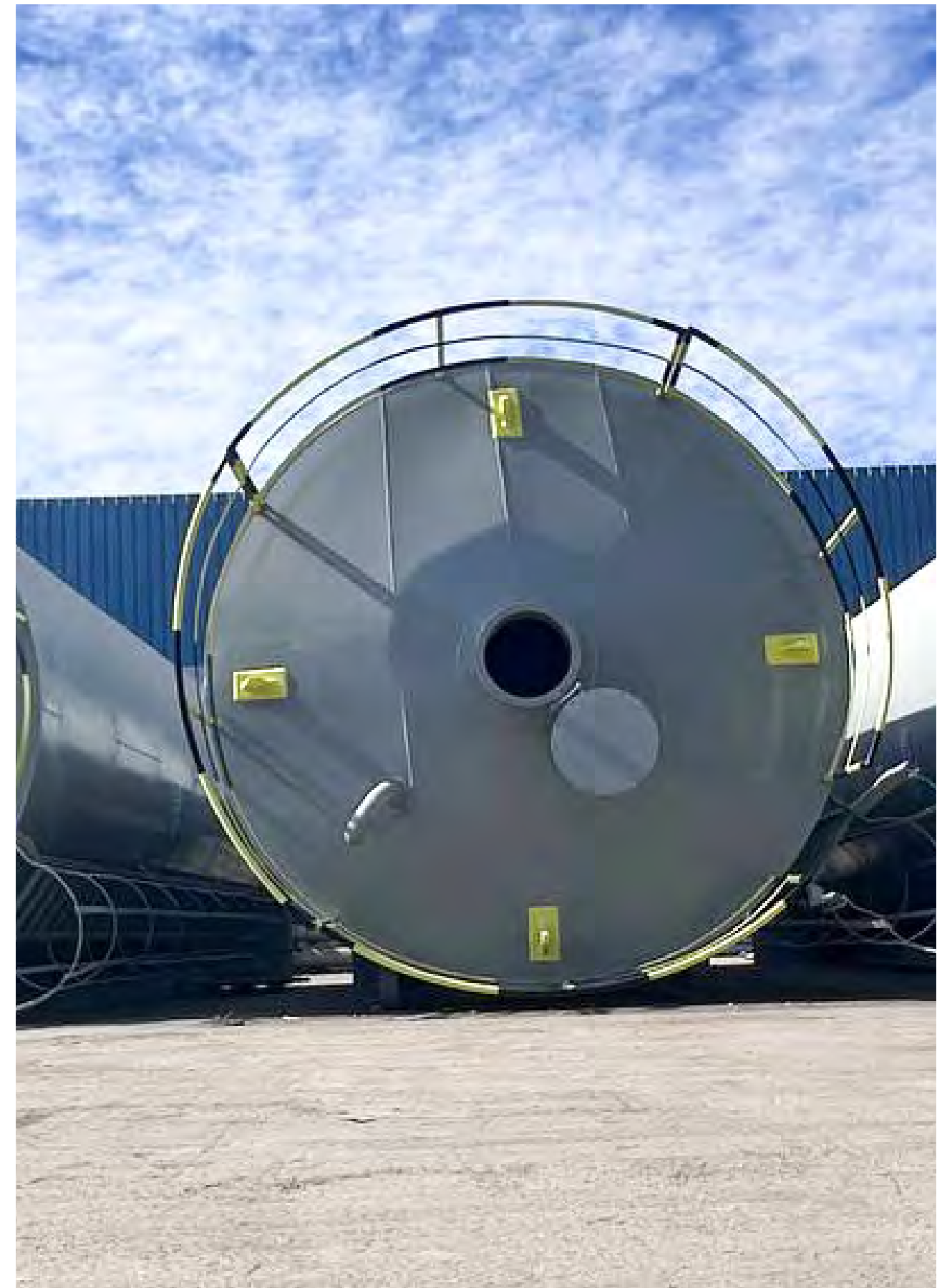
Client: Supplied to Halliburton GSF Scope: Supply, fabrication & epoxy painting of 750 BBL Storage Tanks with handrail and ladder Total Quantity: 494 Tonnes
